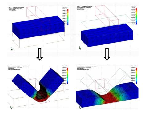
In the example shown above, there are adaptive parts: the top one contacts with a very sharp tool so that a smaller mesh size is needed to well represent the contact surface and better simulate the local large deformation; the bottom part has much smoother profile of material deformation so that the less frequent adaptivity and larger mesh size are used to
