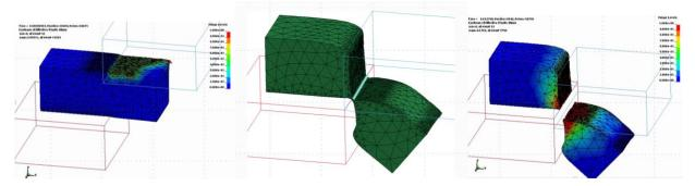
In the metal cutting simulation shown above, it can be estimated when the tool front meets the bottom die so that the additional adaptive step can be triggered for users to trim the mesh using CAD software and then continue the analysis in LS-DYNA.
