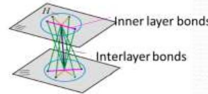
The elastic matrix of laminate material can be **decomposed** to two parts:
