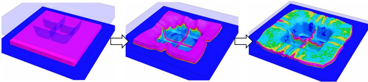
Figure 16: Temperature distribution of the matrix calculated from the thermal conductivity analysis
