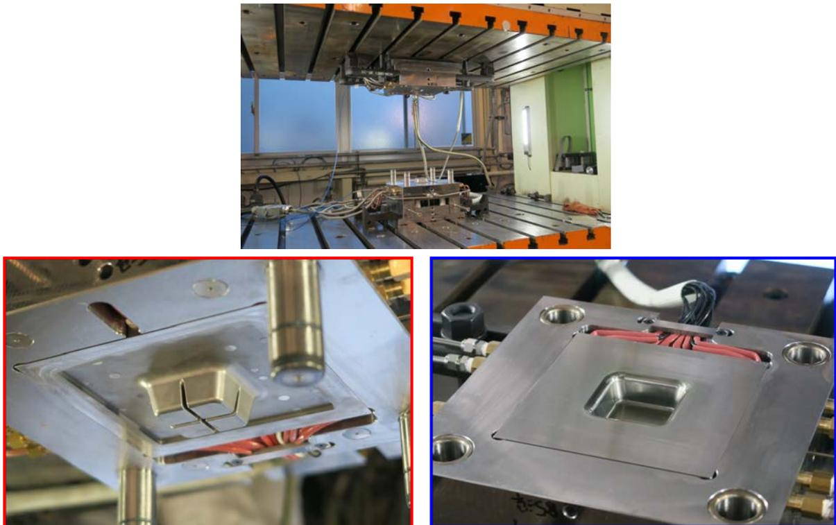
Figure 13: Punch and die shapes used in experiment
