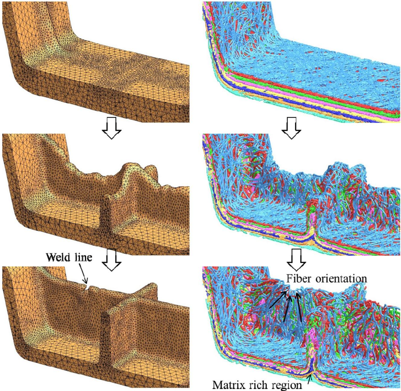
Figure 11: EFG r-adaptive mesh refinement and beam orientation behaviour
