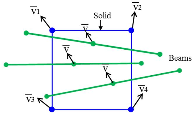
Figure 3: Constraint of multiple beam elements in one solid element
