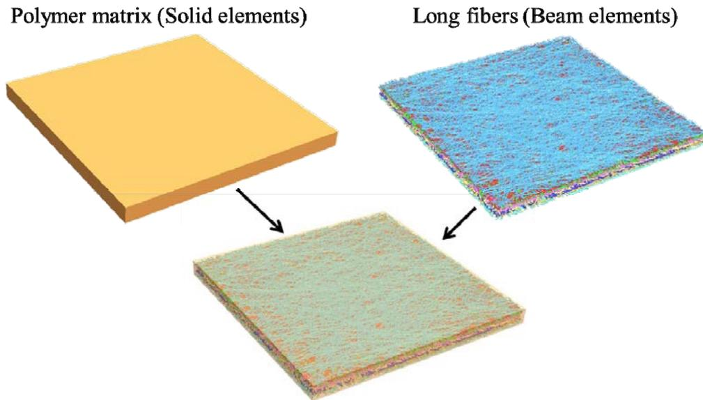
Figure 8: Polymer matrix by solid elements and Long fibers modelled by beam elements
