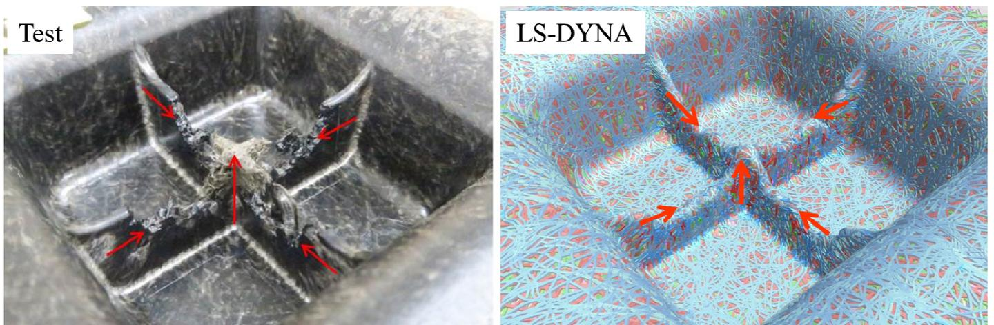
Figure 15: Formation of ribs and weld lines near the final punch stroke
