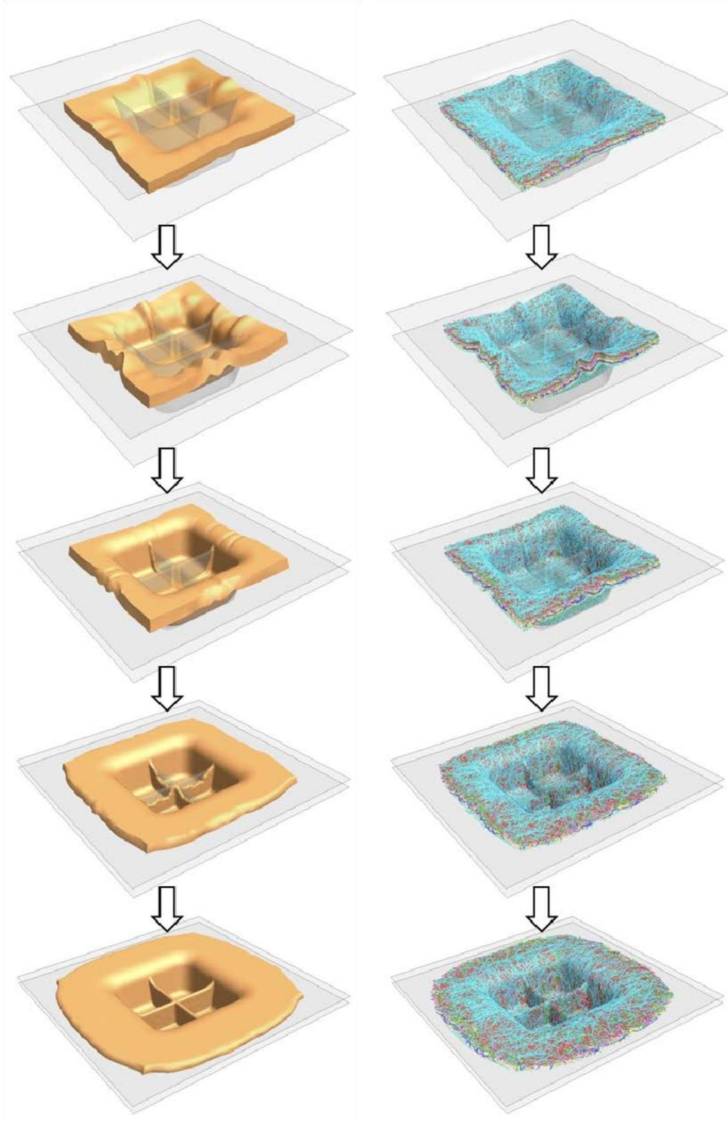
Figure 10: Deformation behaviour of solids as matrix (left) and beams as fibers (right)
