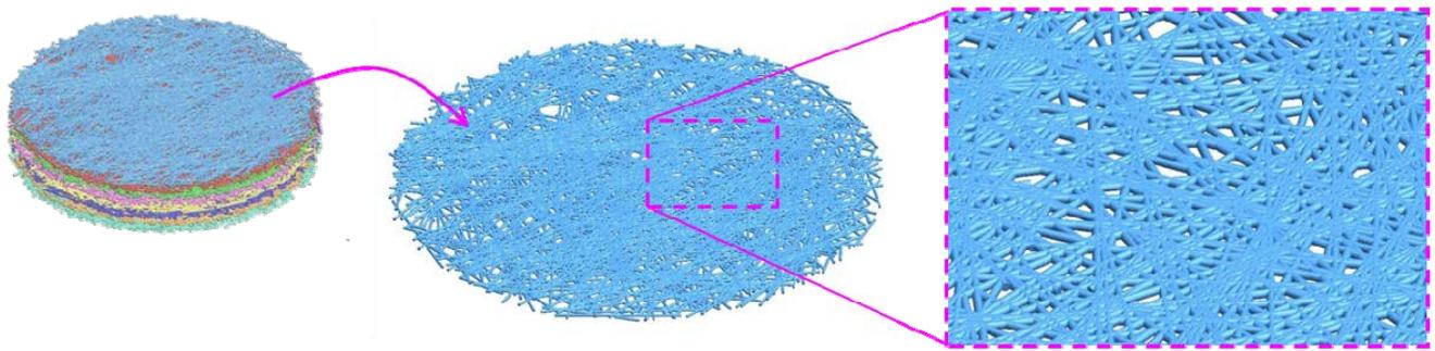
Figure 5: Eight layer model made of beam elements with 2D random orientation
