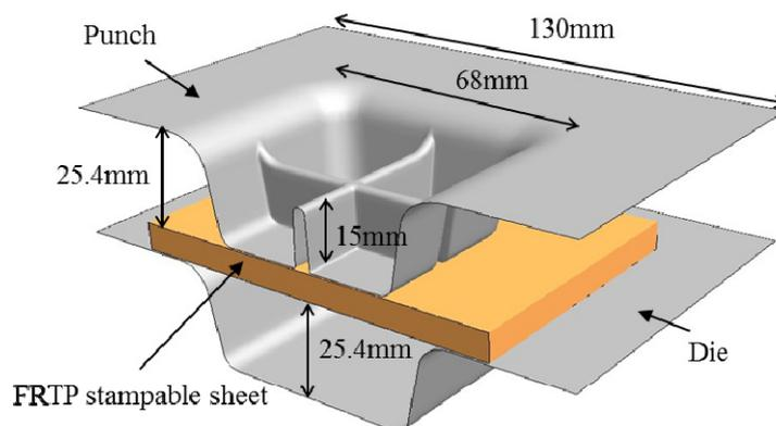
Figure 9: Compression molding model to form cross-rib shaped component
