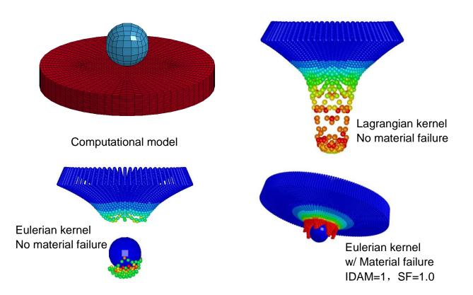
The following shows analysis results of metal cutting and shearing problems using SPG.
