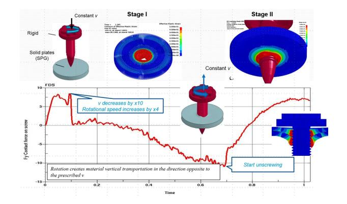
Friction Stir Drilling (FDS) is a very challenging problem for numerical simulation. The conventional methods such as element erosion have difficulty to capture the drilling threads, while adaptive re-meshing is very expensive especially when material failure is taken into account. The above figure shows that, by using SPG (IDAM=1), we can not only well capture the formation of the drilling threads but also successfully simulate the pull-out process.
