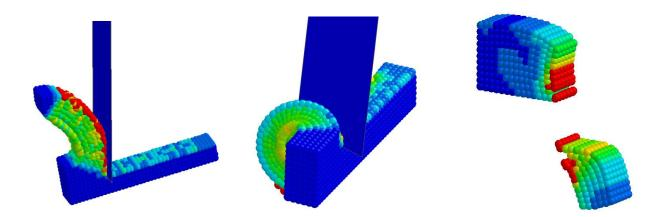
The next plot shows the riveting analysis using SPG, where both plates are modeled by SPG particles.
