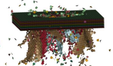
Ball impact on CFRP (Peridynamics)
