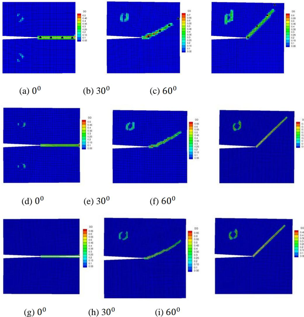
**Fig. 3.** Comparison of experimental (▲) and numerical crack paths for different meshes: (a)-(c) coarse mesh, (d)-(f) medium mesh, (g)-(i) fine mesh; and different fiber orientations (background: inner-layer damage).
