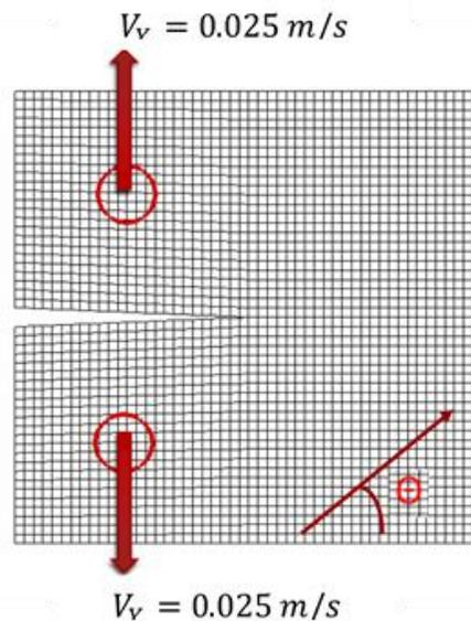
**Fig. 2.** Compact-tension test of a cortical bone plate.
